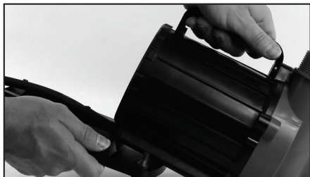
Step 13: Re-fit the base plate.
