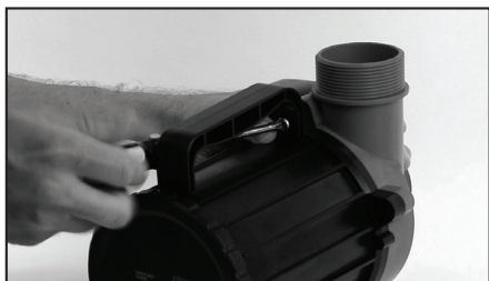
Step 5: Unscrew the screw that is attached to the handle.
