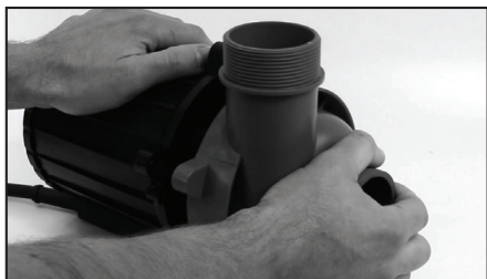
Step 7: Carefully pull away the impeller housing.
