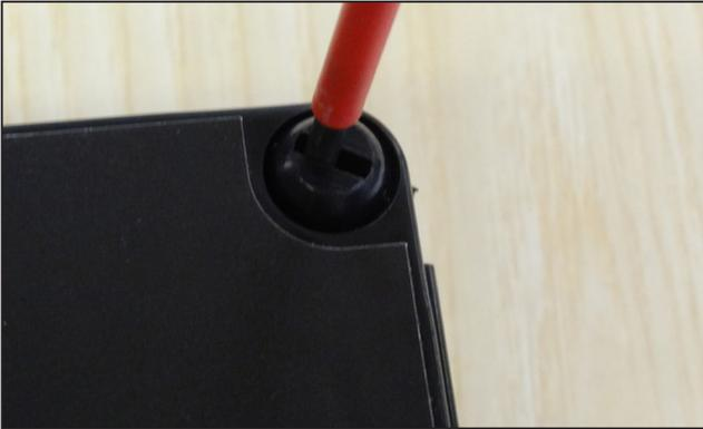
1. To open the box, use a flat head screwdriver to unscrew the plastic screws on the box. The lid can be open to 90° with 2 loose screws. **DO NOT FORCE THIS OPEN.**
